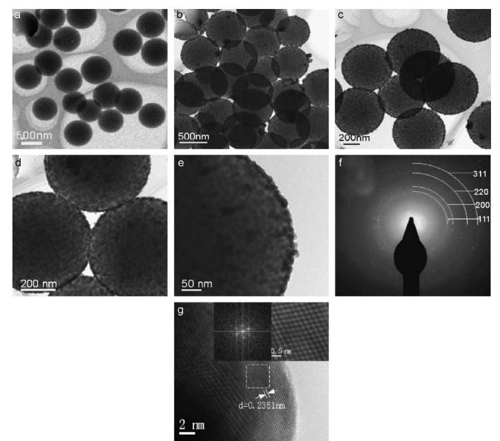
Fig. 2. (a) TEM image of the silica spheres before the coating; (b)–(e) TEM images with different magnifications; (f) SAED pattern of the entire SiO<sub>2</sub>/Ag composite particle corresponding to (e); and (g) HRTEM image of the sample obtained when *I*, *C* and *t* were  $2 \text{ mA/cm}^2$ ,  $3.25 \times 10^{-6} \text{ mol/l}$  and 30 min, respectively.
