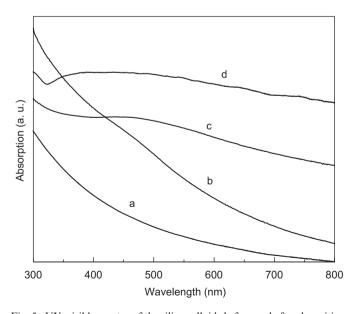
Fig. 5. UV–visible spectra of the silica colloids before and after deposition of silver nanocrystals (a) uncoated silica spheres; (b) silica spheres coated with uniform and isolated silver nanoparticles (as shown in Fig. 4a); (c) silica spheres coated with a silver layer of  $14\pm 2$  nm in thickness (as shown in Fig. 2); and (d) silica spheres coated with a silver layer of about 20 nm in thickness (as shown in Fig. 4c).
