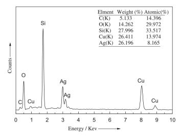
Fig. 3. EDX analysis of the silica spheres coated with a silver layer of  $14\pm 2$  nm in thickness.
