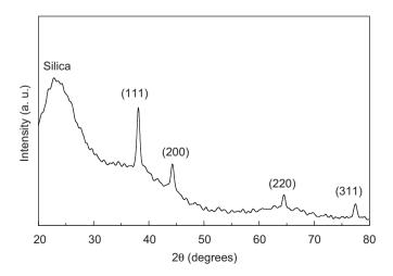
Fig. 1. XRD pattern of the sample synthesized when *I*, *C* and *t* were  $2 \text{ mA/cm}^2$ ,  $3.25 \times 10^{-6} \text{ mol/l}$ , and 30 min, respectively.
