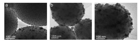
Fig. 4. TEM images of the samples synthesized when *I*, *C* and *t* are, respectively (a)  $0.75 \text{ mA/cm}^2$ ,  $3.25 \times 10^{-7} \text{ mol/l}$  and 30 min; (b)  $2.5 \text{ mA/cm}^2$ ,  $3.25 \times 10^{-6} \text{ mol/l}$  and 30 min; (c)  $2.0 \text{ mA/cm}^2$ ,  $3.25 \times 10^{-4} \text{ mol/l}$  and 30 min.
